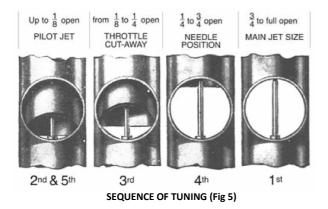
**NOTE.** The carburetor is automatic throughout the throttle range - the air valve should always be wide open except when used for starting or until the
