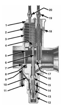
Fig. 2 - Section through mixing chamber
